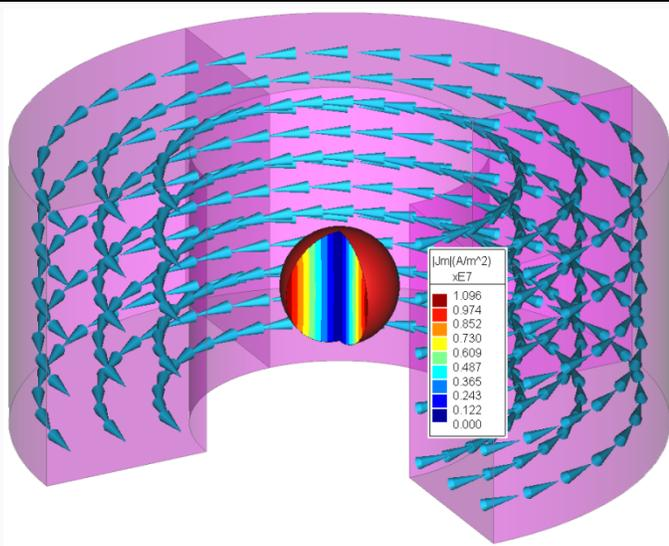
We will use the electromagnetic solution to obtain the steady-state electrical power transferred to the sphere and also examine the transient start-up conditions that occur when the coil is first energized.
