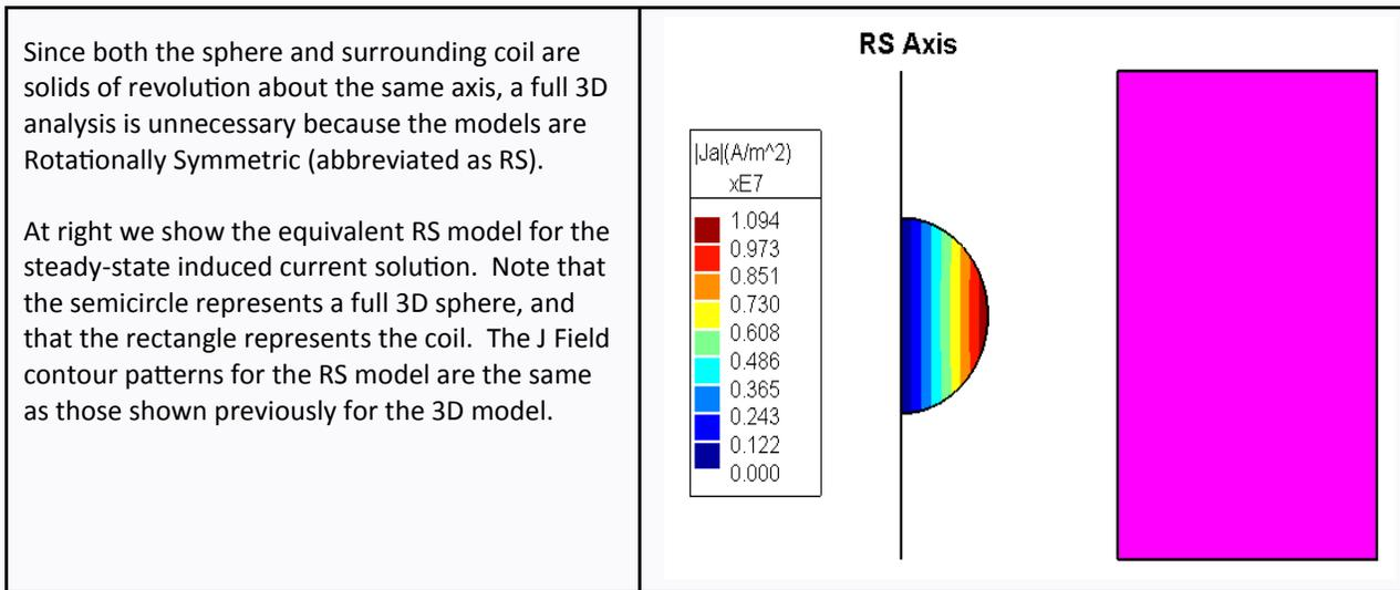
Because of the Rotational Symmetry, the field solutions are equivalent to full 3D models. We will use this fact to our advantage and display simulation results for RS models throughout the rest of this paper.
