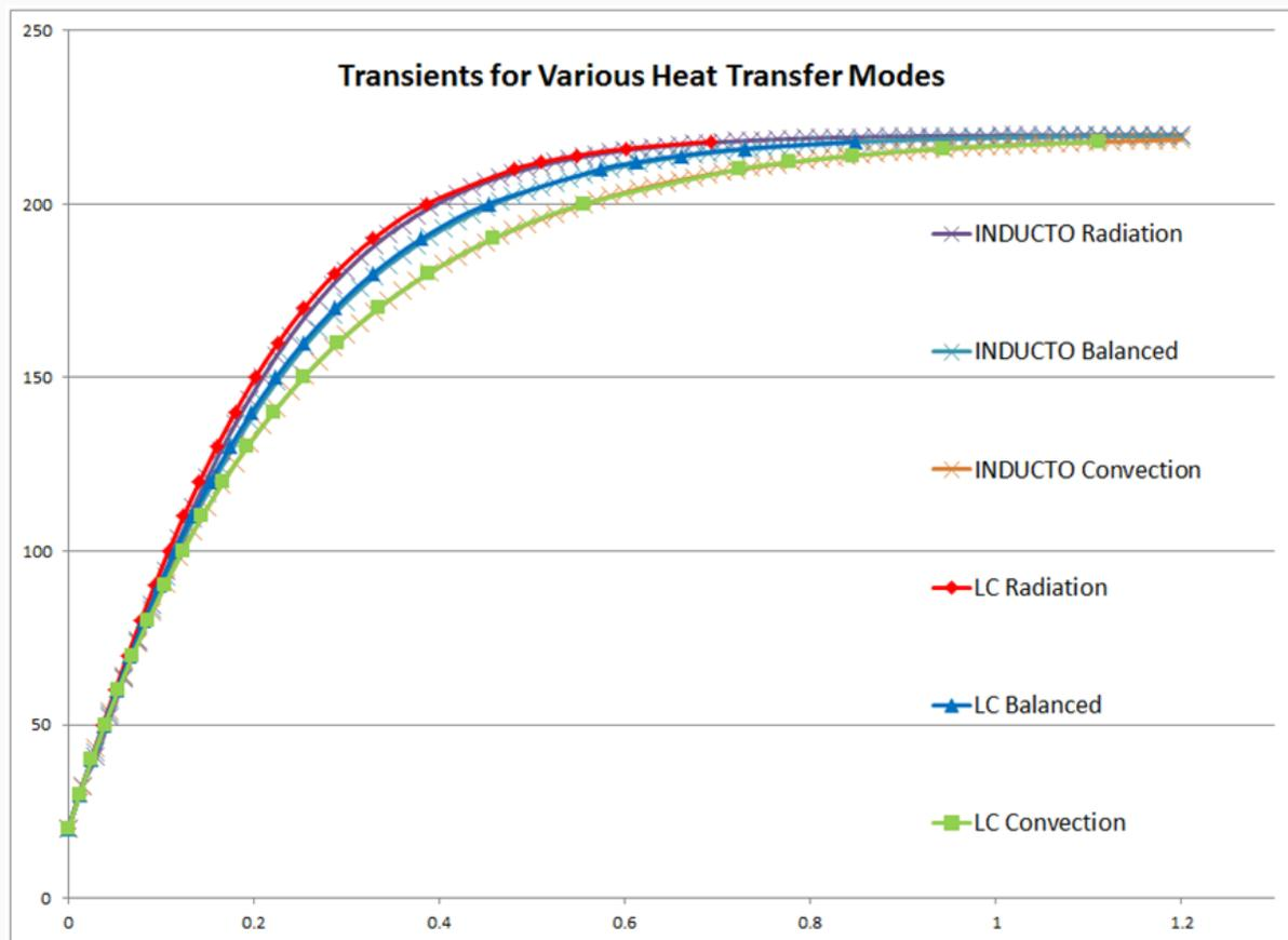
It is interesting that heat transfer by radiation produces the fastest transient.
