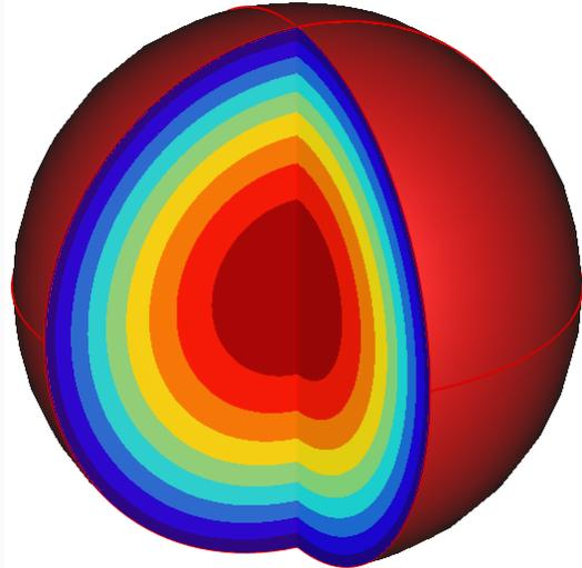
Our electromagnetic model will utilize the same sphere with the addition of a surrounding coil carrying 60 Hz current.
