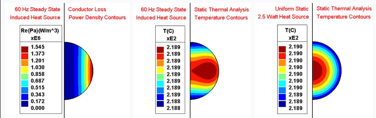
The temperature contours produced by the uniform volume heat source are simple concentric spheres, but the non-uniform eddy current heating produces a more complex distribution.
