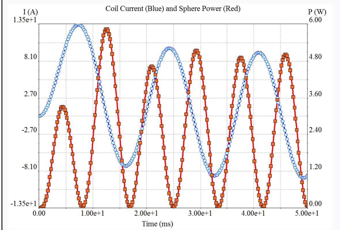
Note that the steady-state power loss is a time varying signal. In fact it is the sum of a constant average value plus a **120 Hz** sinusoidal signal. It can be shown mathematically that the power signal for linear systems will always oscillate at *twice* the frequency of the current (or voltage) signals.
